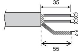
Length of stripped digital Input/Output communication wire
