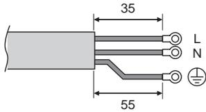
Attach a round pressure terminal to the end of each wire of the power cable, communication cable and power cable for central controller.
